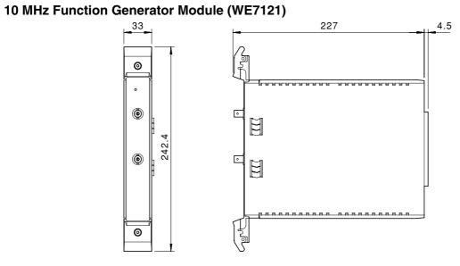
If not specified, the tolerance is  $\pm 3\%$  . However, in cases of less than 10 mm, the tolerance is  $\pm 0.3$  mm.
