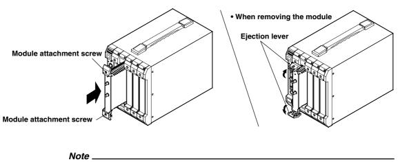
When synchronizing output signals from multiple function generators, install the modules in adjacent slots.
